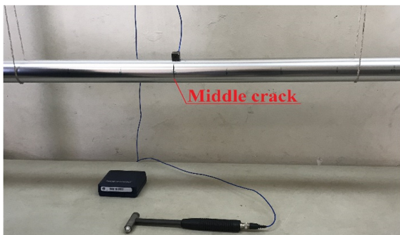
Fig. 20 Setup modal analysis of cracked pipe
