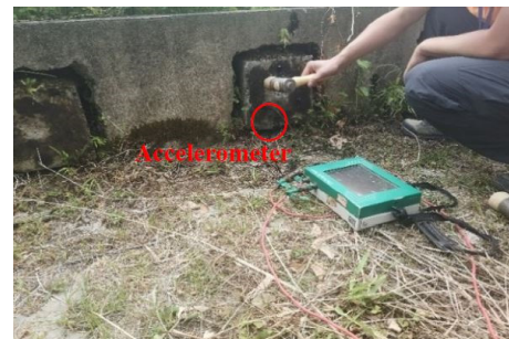
Fig. 18 The setup of the pile test
