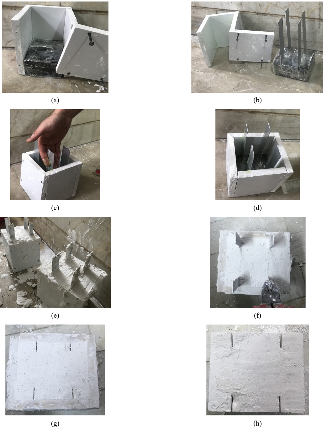
Fig. 2 (a) A special black plastic fiber with dimension of 10\text{ cm} \times 10\text{ cm} \times 5\text{ cm} was put into the frame; (b) the shime inside the plastic fiber; (c) Grace around the shime; (d) adjustment the shime inside the frame; (e) plaster slurry inside the mold; (f) the aluminum sheet is removed from the mold; (g) the specimen consisting non-persistent crack inside the frame; (h) the specimen consisting non-persistent crack outside the frame
