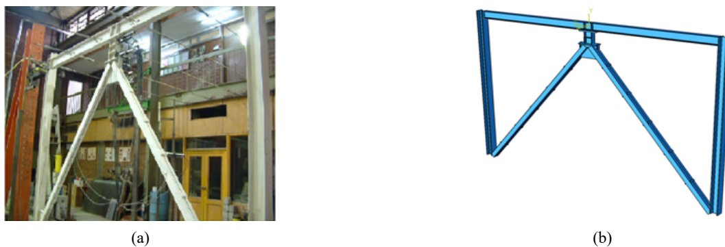
Fig. 6 (a) Experimental specimen (Zahrai 2015); and (b) numerical model
