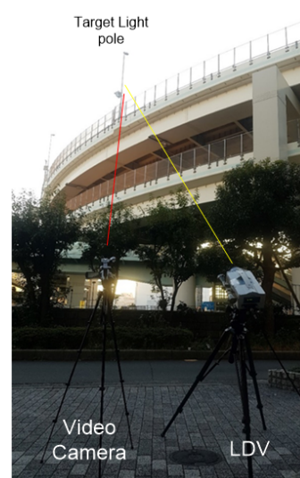
(b) Experimental setup with LDV and high-speed video camera system
