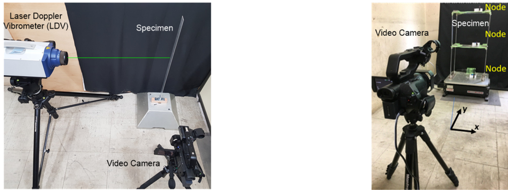
(a) Setup for cantilever beam experiment with LDV as reference
