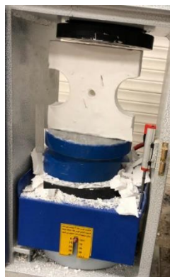
Fig. 4 Specimen are placed between the plates of the loading machine
