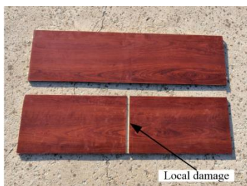
(a) Damaged and undamaged plywood plates
