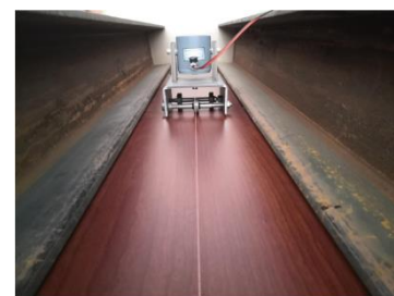
(c) The plywood plate is detected by an actively excited vehicle under the action of the traction motor
