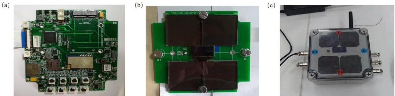
Fig. 7 Components of the monitoring station (MS). (a) PCB circuit board; (b) micro solar panel; and (c) complete monitoring station after assembly
