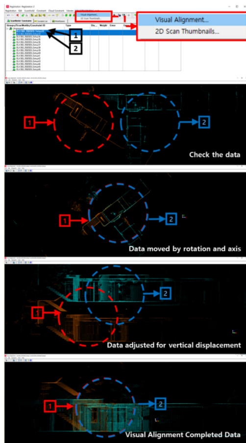
(a) Visual Alignment adjustment process
