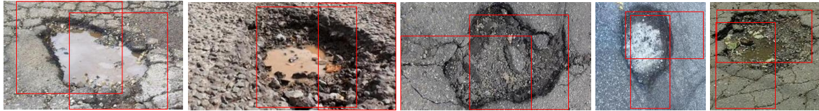
Fig. 8 Examples of one pothole detected as multiple potholes with overlapping bounding boxes
