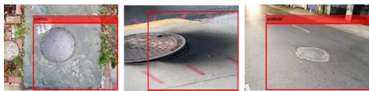
Fig. 15 Few manholes falsely classified as potholes
