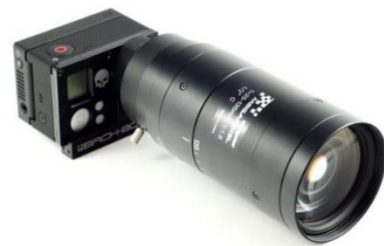
Fig. 1 Modified Action Camera with Zoom lens and synchronization hardware attached
