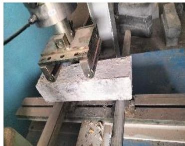
(c) Flexural test
