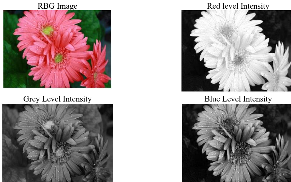
Fig. 14 RGB picture with all 3 colour matrices shown and split into each colour matrix (Wilbur, 2011)
