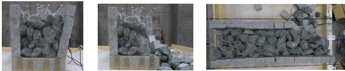
(a) Stone arch bridge with large crushed stones excited by sine wave with frequency of 6 Hz and amplitude of 150 gal
