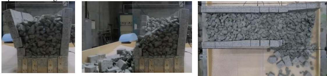
(d) Stone arch bridge with small crushed stones excited by sine wave with frequency of 33 Hz and amplitude of 150 gal
