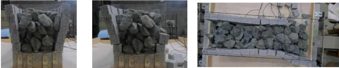
(c) Stone arch bridge with large crushed stones excited by sine wave with frequency of 33 Hz and amplitude of 150 gal
