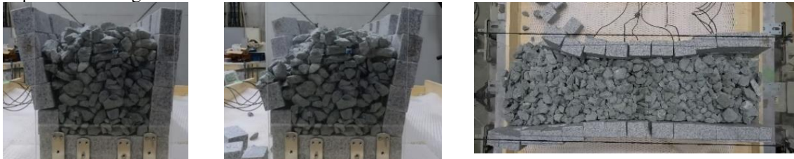
(b) Stone arch bridge with small crushed stones excited by sine wave with frequency of 6 Hz and amplitude of 250 gal
