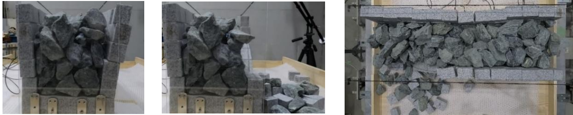
(a) Stone arch bridge with large crushed stones excited by sine wave with frequency of 6 Hz and amplitude of 250 gal
