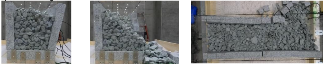
(b) Stone arch bridge with small crushed stones excited by sine wave with frequency of 6 Hz and amplitude of 150 gal
