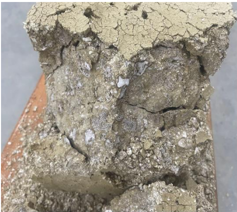
Fig. 6 Morphology after 1 day of standing at 900°C
