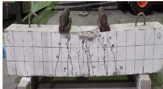
Fig. 27 Deflection and plastic strain in Concrete Beam C3
