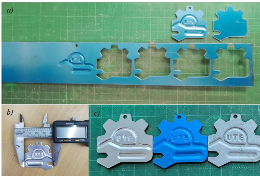
Fig. 11 Results from the forming experiment. a) initial blank and the stamped part, b) dimensional inspection, and c) final product."
