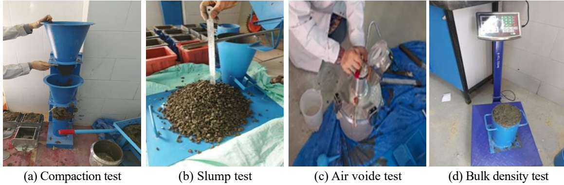
Fig. 9 the steps of slump and compaction test
