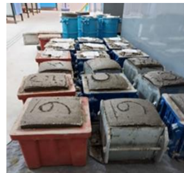
(b) Samples tested cubes RC
