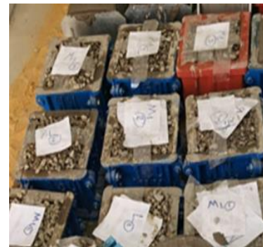
(b) Samples tested cubes RC
