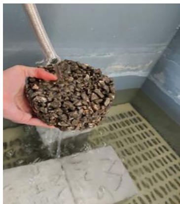
(a) Concrete Porous
