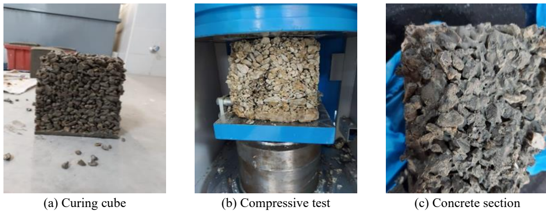
Fig. 18 Compressive Test for First Group [RC]
