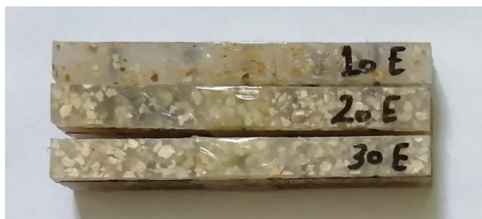
Fig. 4 Eggshells composites before flexural test
