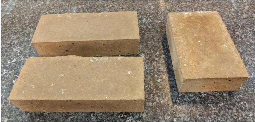
Fig. 1 Samples of geopolymer brick made based on sand washing waste powder with sand filler
