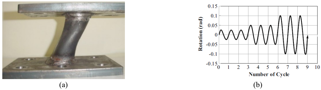
Fig. 1 Experimental test of CFSD by Abebe et al. (2019): (a) specimen deformed shape and (b) cyclic loading protocol
