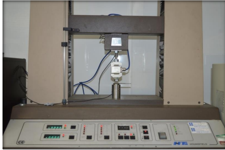
Fig. 2 Setup of the instrumented facility used for quasi-static testing
