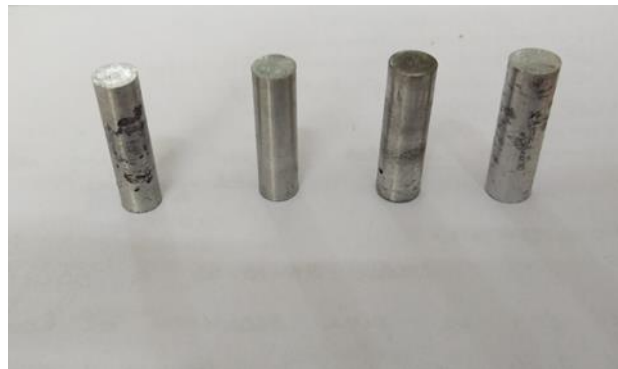
Fig. 3 Specimens of Al8090/TiB 2 /C composite used for wear test
