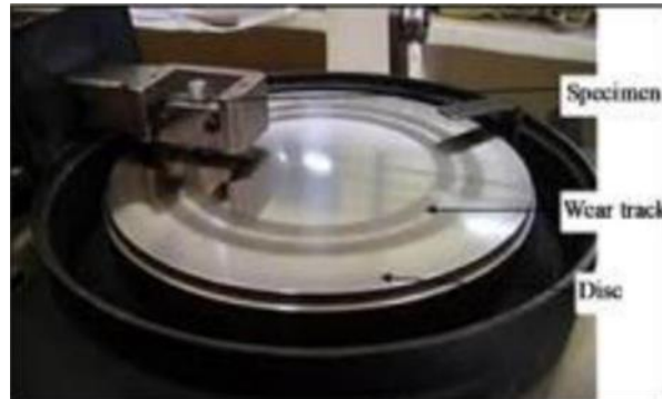
Fig. 2 Tribometer testing setup for wear analysis
