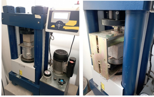
Fig. 3 Experimental device for compression test on the left and splitting tensile test on the right
