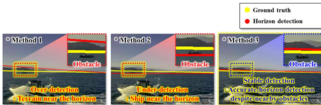
Fig. 14 Results of three methods for horizon detection in complex maritime environments with terrain and ships
