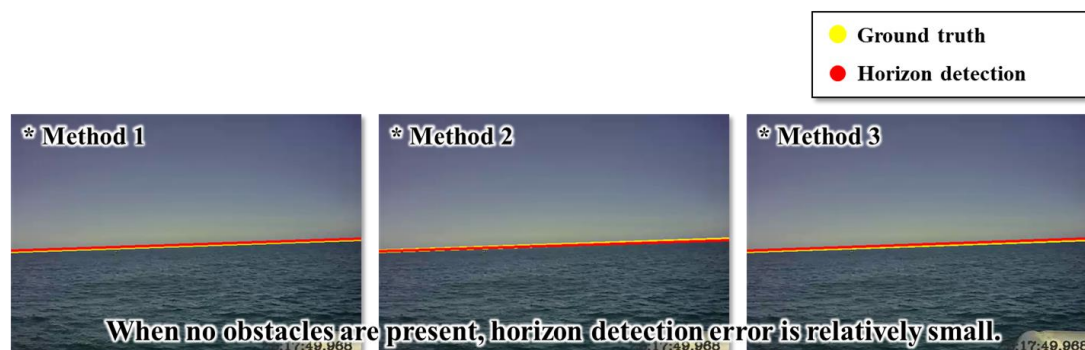
Fig. 12 Results of the three methods for horizon detection in simple maritime environments
