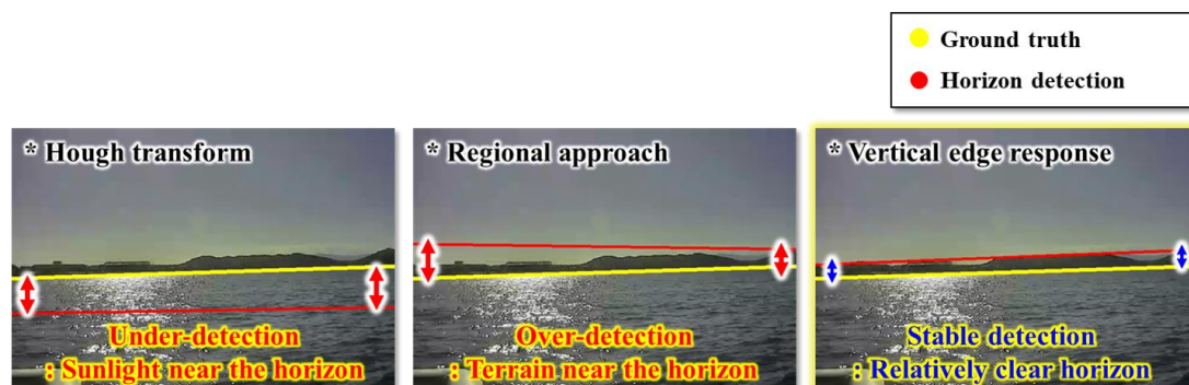
Fig. 10 Results of three methods for horizon edge classification
