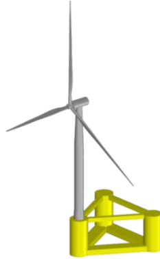
Fig. 3 Schematic of 15 MW FOWT Model
